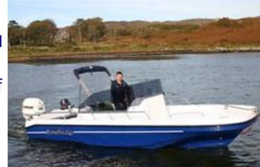
The latest launch is the **Stormbreaker 710 Tourer** using a proven cathedral hull design of the Stormbreaker with the same strong handling abilities in rough weather. In response to customers needs we have added an "A" frame and canopy which means she can be used all year round. Performance has not been compromised with a speed of 44 knots. Stormcats is now an authorised Yamaha and Tohatsu dealer and can purchase engines, spare parts and carry out servicing at a competitive rate.
